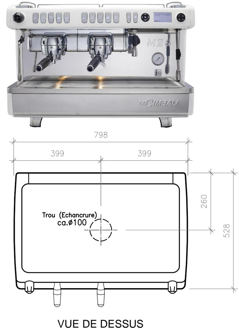
PLAN DE RACCORDEMENT POUR LA MACHINE A CAFE M26 TE RE 3-gr.
