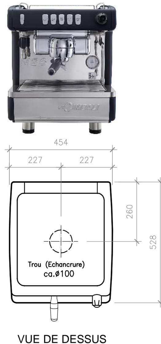
PLAN DE RACCORDEMENT POUR LA MACHINE A CAFE M26 TE RE 2-gr.
