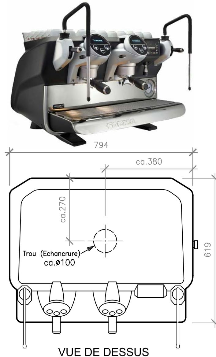
PLAN DE RACCORDEMENT POUR LA MACHINE A CAFE E-71E 3-gr.
